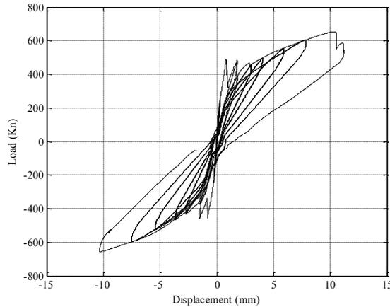
Figure 4. Cyclic Response of SW2 at Axial Load Ratio of 5%
