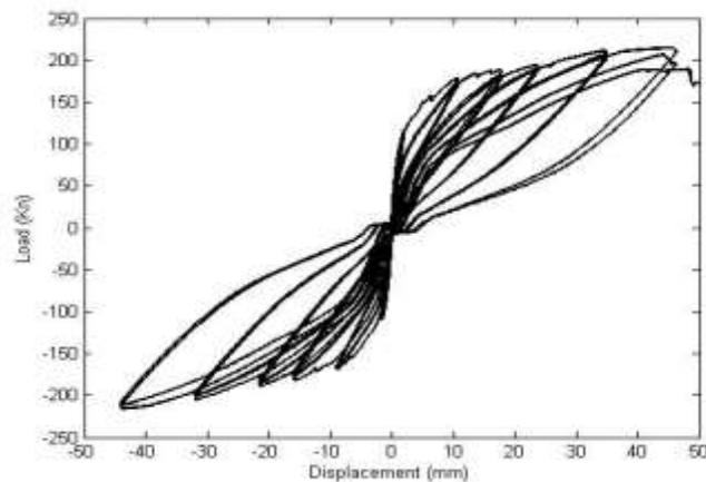
Figure 7. Cyclic Response of IW3 at Axial Load Ratio of 5%
