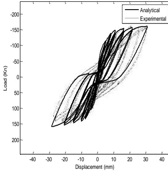
(b) Steel RC Intermediate Wall
