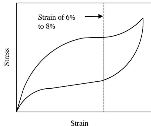
Figure 1. Typical Stress-Strain Response of SMA Reinforcement
