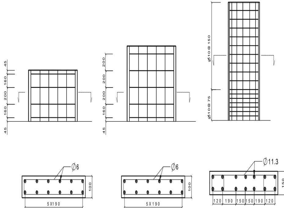
Figure 3. Reinforcement Details for Squat and Intermediate Walls (Dimensions in mm)
